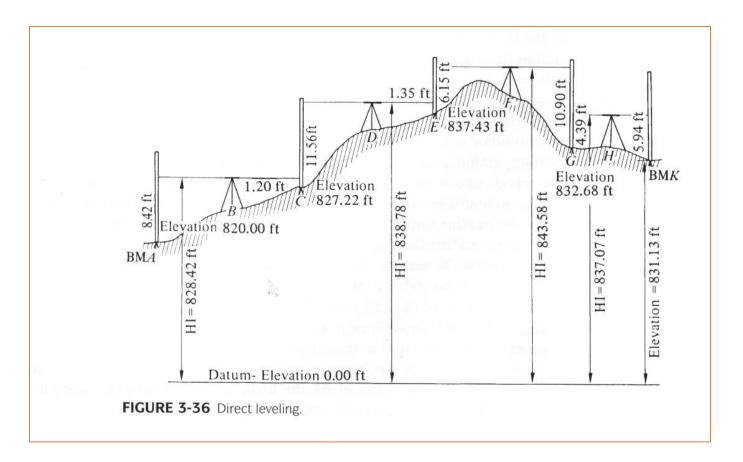
Height differences between the consecutive locations of backward and forward rods correspond to the local separation between the level surfaces through the bottom of the rods, measured along the plumb line direction
