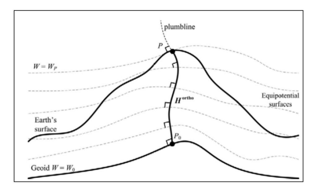
Figure (1.5): The orthometric height (H <sup>ortho</sup>) of P [2].
