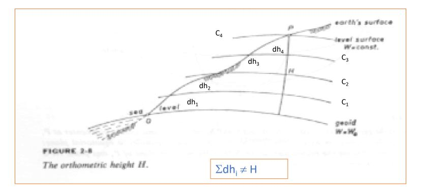
$C_1$ ,  $C_2$ ,  $C_3$ ,  $C_4$  – geopotential numbers corresponding to level (equipotential) surfaces  $dh_1$ ,  $dh_2$ ,  $dh_3$ ,  $dh_4$  – height difference between the level surfaces (determined by spirit leveling, path-dependent); their sum is not equal to H !
